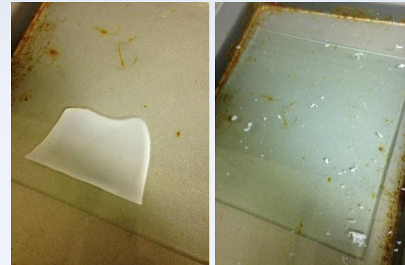
Membrane fabrication using NMP (left) and DMF (right) as solvent.
